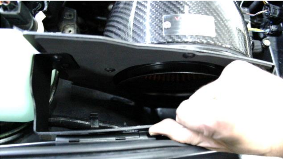
37. As you move the intake down – push back the bracket on the front of the intake to clear the wing. It needs to sit over the sensor – see next step.
