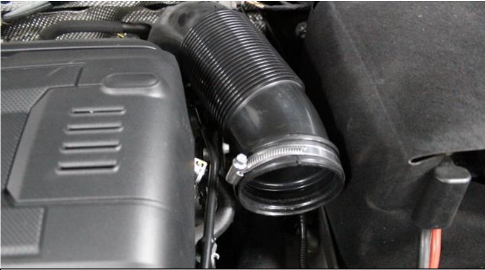
16. Place the supplied hose clamp around the stock inlet tube.
