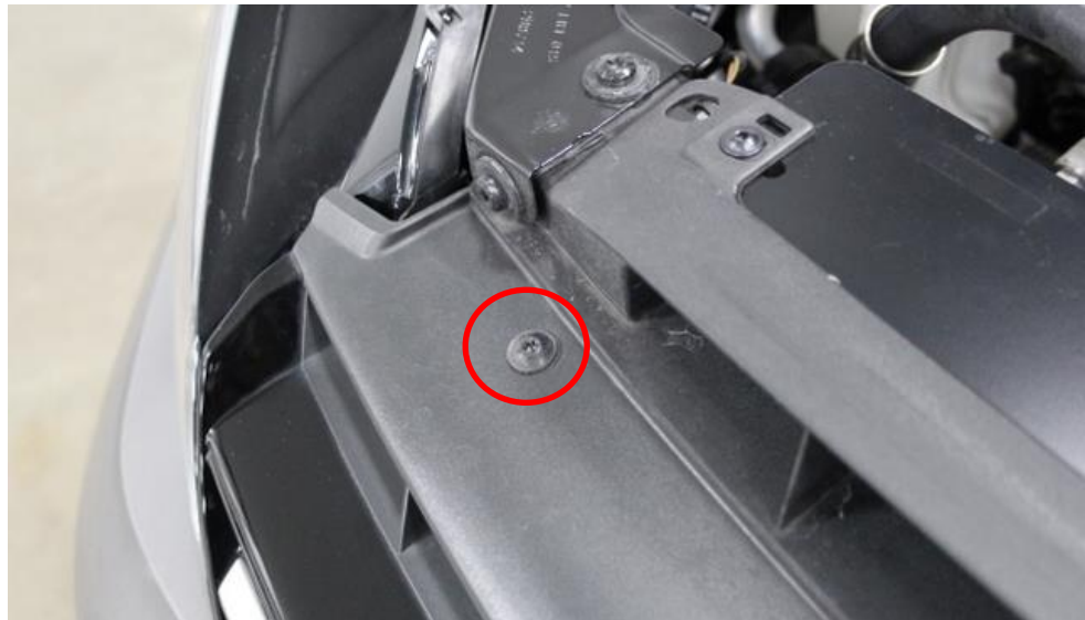
35. Secure both sides with the screws removed from step 23.
