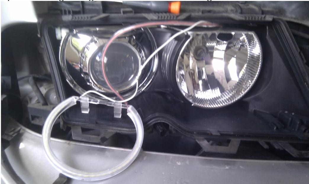
6. When both rings are on and wires routed to the back, test them again to make sure the connections are working.
