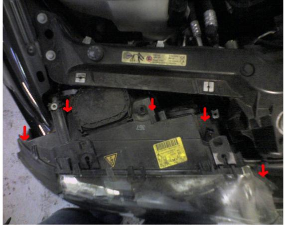
Remove headlight washer trim and cover (if applicable) and pull headlight away from the car. Use a hair dryer to soften the sealant and pull headlights apart. Make sure you remove the remaining screws on the back of headlights so the lense can be pulled away from the housing.
