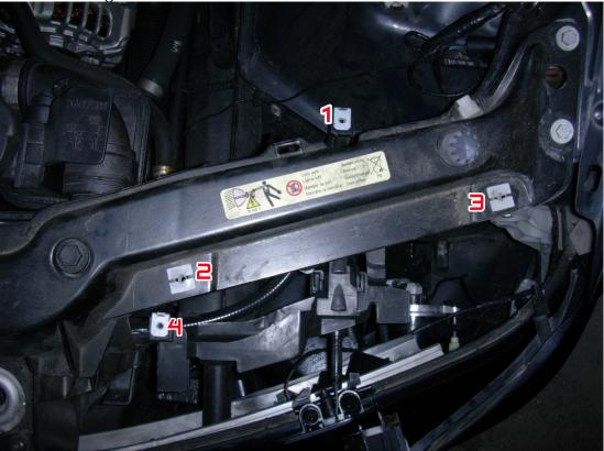
Remove 4 screws and unplug cables and connectors
