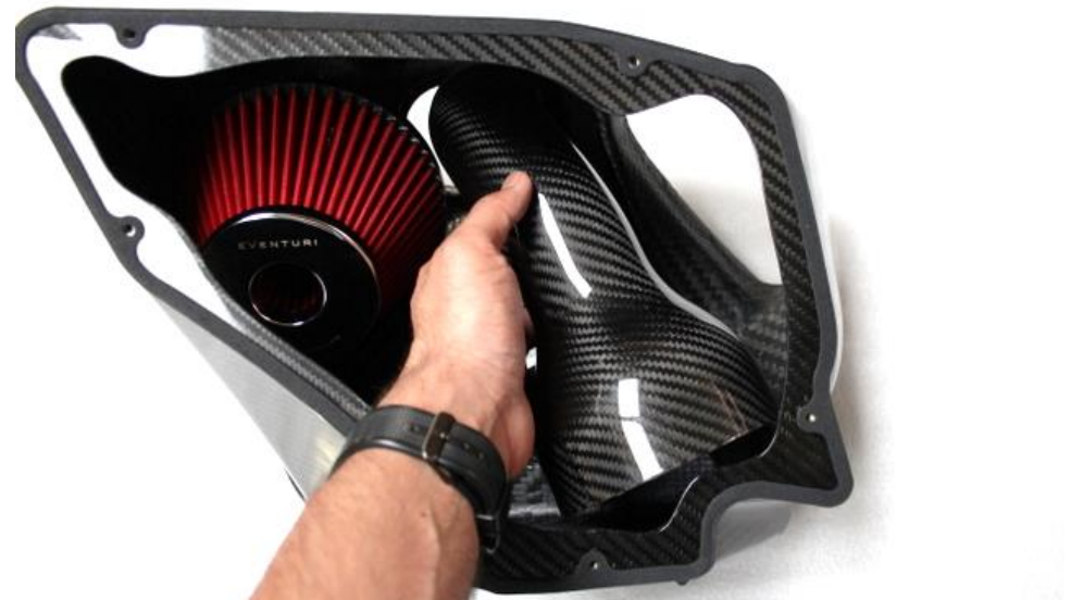
20. Take the longer tube and carefully place into the airbox – push the tube through the hole.
