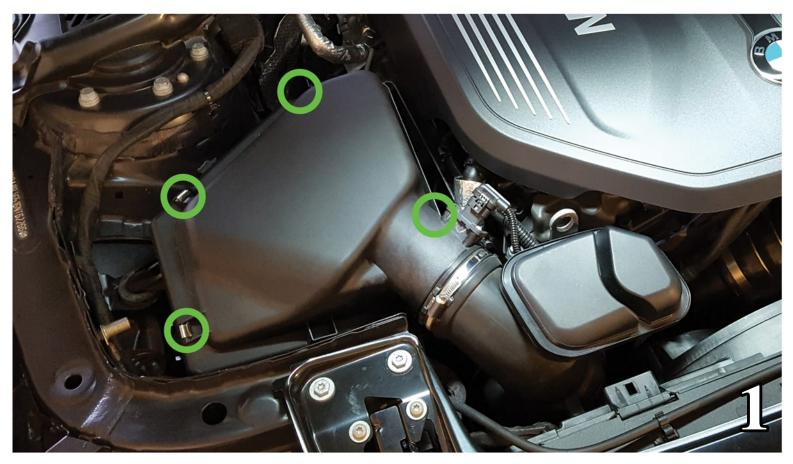
1. Unclip the 4 silver clips on each side of the factory air box lid with a flat head screwdriver by prying away from the air box. They are circled in green in photo 1.
