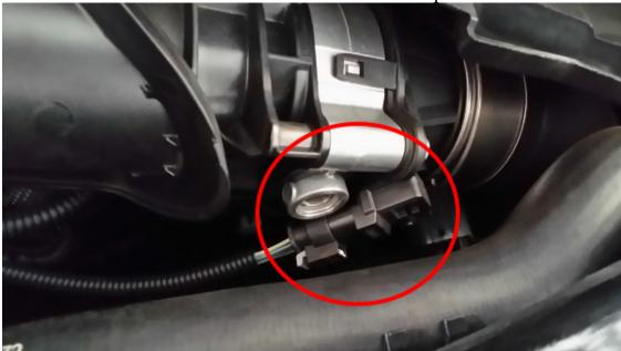
3. Unplug the factory plug by pressing down the tab or by using a small screwdriver on the back side to lift up the clip from the back and sliding the connector off the sensor. Plug the factory sensor wire in to the JB+ and plug the JB+ in to the sensor.
