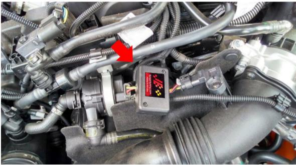
4. Installation is complete! Your car will adapt to the JB+ over a few racing cycles. For the B58 model we suggest tucking the JB+ unit under the plastic engine cover as much as possible.
