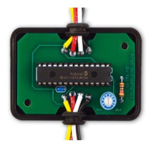
The JB+ is adjustable from 0psi over stock to 4.5psi over stock using the white adjustment dial. Adjustment is made using a small screwdriver to turn the white inner dial. Do not turn the entire blue pot or you may damage the JB+. Towards the "max" setting indicates more boost "min" setting indicates less boost. The default setting of 3pm on the dial is ~4psi over stock.
